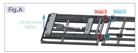
a. Lift the frame slightly and insert a short bolt through the hole in the hinge of the frame. (Refer to the blue indicators in Fig.A)
