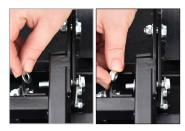
c. If the bolt holes are not aligning, there are two hinge movements that need to be adjusted. Adjust both directions while inserting the bolt to find alignment.
