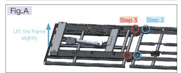
a. Lift the frame slightly and insert a short bolt through the hole in the hinge of the frame. (Refer to the blue indicators in Fig.A)
